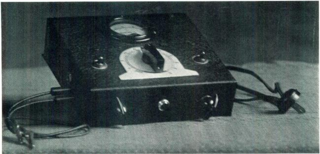
The dial scale is hand-drawn on bristol board and cemented to the panel.
