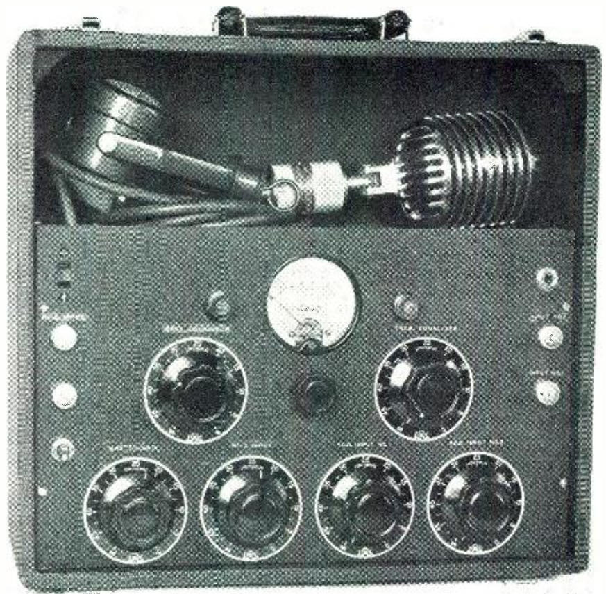
Mikes and cables are carried in the compartment above the amplifier unit. Incoming cables are kept clear of the various gain and equalizer controls.
